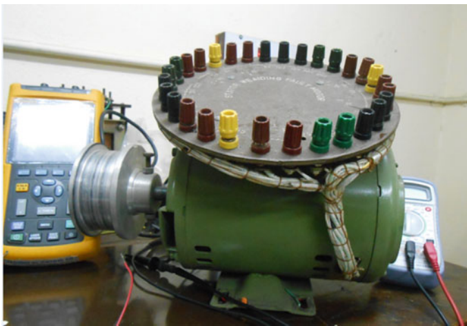
Fig. 6.3 Induction motor, used for the experiment (courtesy Power System Lab, Department of Applied Physics, University of Calcutta, India)
